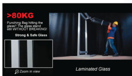
> 80KG Sandbag Stress Test
