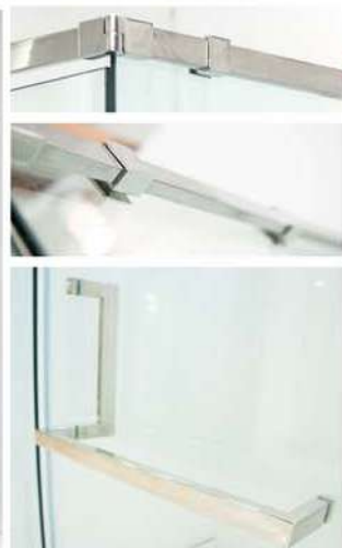
Model: REH100 SQ / Finish: Stainless Steel Glossy Polish G.Thickness: 10mm Clear Tempered / Header: S.Steel 304
