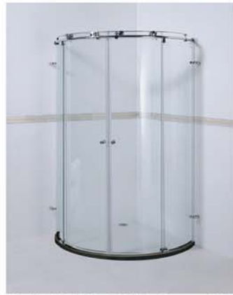
Model: KK-T41 - 2 Sliding Door + 2 Fix Material: Full SUS304 Stainless Steel G.Thickness: 8mm Clear Tempered Size: 985 x 985 x 2000mm H
